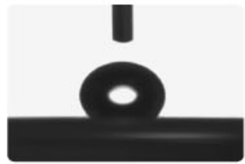
ReDura™ of > 90° contact angle with hydrophobic surface property
